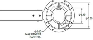
CAMERA MOUNTING LIMITATIONS 3 OR 4 -HOLE MOUNT 3.4" DIA. TO 5.65" DIA. UNITS: INCHES
